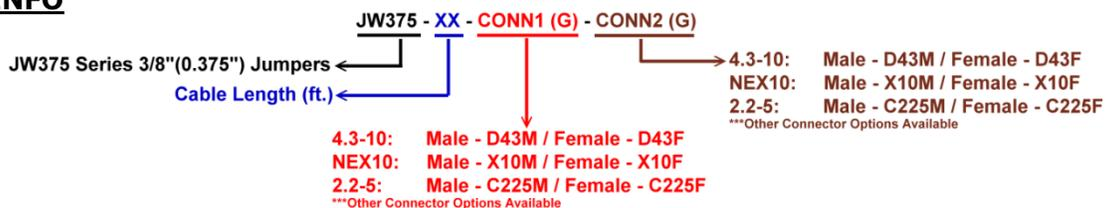
Example: 20 Feet Jumper Cable (w/Boots) with 4.3-10(M) and NEX10(M) Connectors --- PN: JW375-20-D43M-X10M
