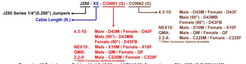
Example: 12 Feet Jumper Cable with 4.3-10(M) and NEX10(M) Connectors --- PN: J250-12-D43M-X10M
