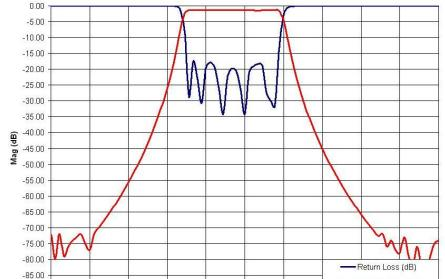
Frequency Range: 2426MHz - 2448MHz (CH6) No. of Cavities: 8 (4 sections also available)
