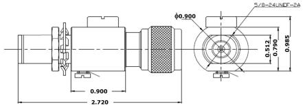
Dimension shown above is for Model#: 321-50-6G-N. Dimensions vary between different Models.
